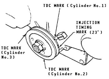
below). Remember the engine's firing order is 1-3-2. You may find that turning the engine's crankshaft is more easily accomplished when the engine's glow plugs are removed before the crankshaft is rotated.
