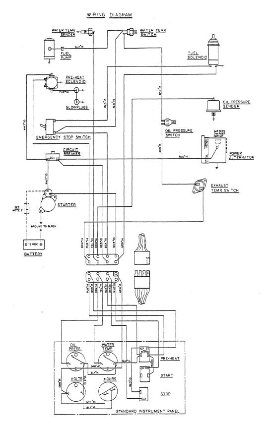
BCD 4.4KW DC Control Circuit Wiring Diagram #35951 page 1 of 2
