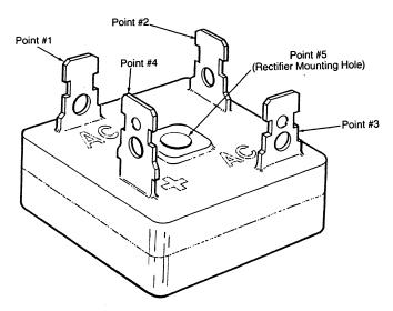
E. Place the positive (+) lead on point #1 and the negative (-) lead on point #3. The Ohmmeter again should not register any deflection (no deflection indicated infinite resistance). Reverse these connections and the Ohmmeter should again register no deflection. IF THE RECTIFIER FAILS ANY OF THE PREVIOUS TESTS (A - E), REPLACE THE RECTIFIER BECAUSE IT IS DEFECTIVE.
