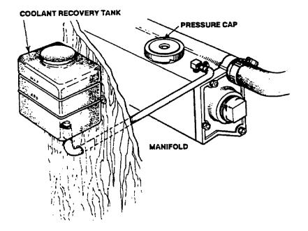
Coolant Recovery Tank, Recommended Installation
