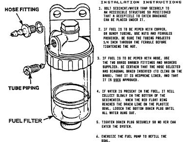
Westerbeke warranty. The owner/operator is responsible in making sure that fuel reaching the engine's injection equipment is free of impurities. This process is accomplished by installing a proper filtration/separation system and maintaining this system.
