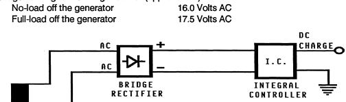
Normal DC voltage running out of the rectifier (in Volts DC) is measured across the two DC connections of the bridge rectifier; that is, + and -.
