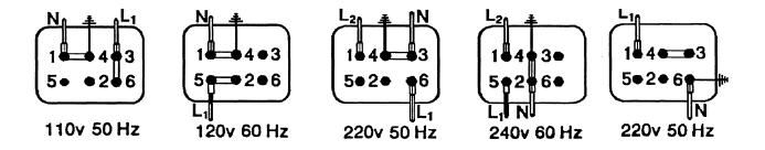
For making connections to the AC terminal block, use terminal ends for #10 studs which will accept multistrand wire sized for the number of conductors in the bundle, the rating of the conductor's insulation, and amperage that will be drawn through the conductor(s). (Refer to the generator's data plate for the generator's amperage and voltage ratings.)
