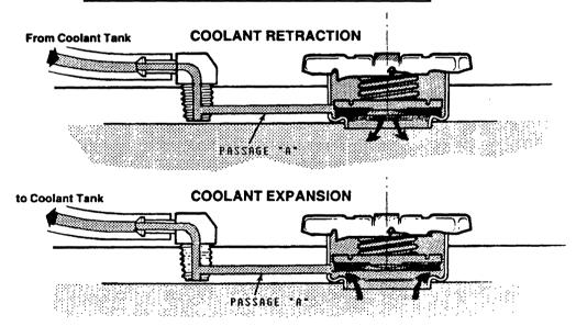
FUNCTION OF MANIFOLD PRESSURE CAP
