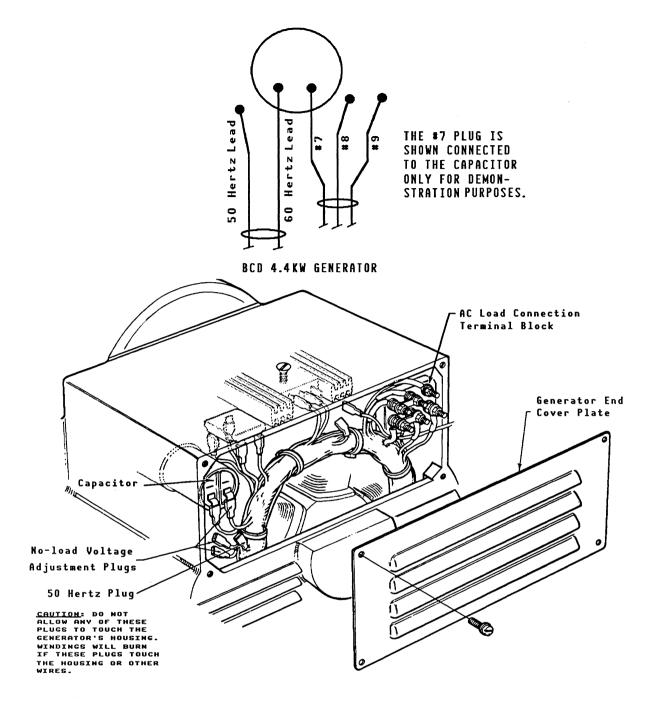
A. Check the resistance of the exciter windings
