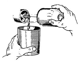
When installing the new oil filter element, wipe the filter gasket's sealing surface on the engine block free of oil and apply a thin coat of clean engine oil to the rubber gasket on the oil filter. Screw the filter onto the threaded oil filter stub, and then tighten the filter firmly by hand.
