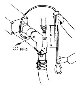
Dry stack-type exhaust systems (shown to the right) must be attached to the generator engine's exhaust manifold by means of a flexible connector pipe. This system must be properly supported and insulated to prevent water from entering into the engine's cylinders. Provisions must be made for discharging the engine's cooling sea water.
